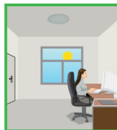
Light will switch off automatically even with presence detected, if the nature light is sufficient.
