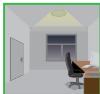
The light still dims to 0/10%/30%/50% if still insufficient natural light, the light never switch off until sufficient natural light.
